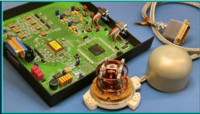
AT: Comet Interceptor DFP Fluxgate magnetometer (EM)
